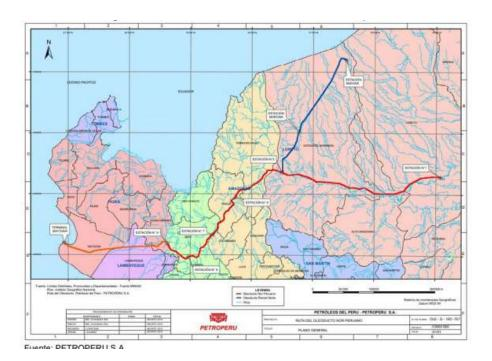
It is important to note that the ONP has a "Reserve Zone," which consists of a strip 75 meters wide on each side of the pipeline axis. This zone was established to ensure the safety and integrity of the infrastructure, forming a total width of 150 meters along its route through the departments of Loreto, Amazonas, Cajamarca, Lambayeque, and Piura<sup>2</sup>.
